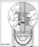
**3.** With the provided spanner unscrew and remove the central rear bolt **A.**
